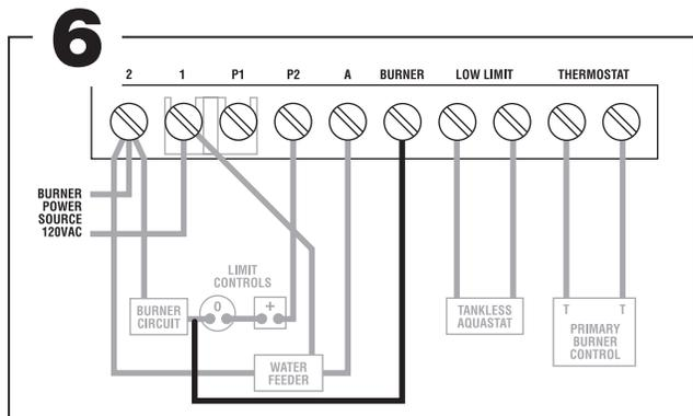
Connect "BURNER" terminal on the CycleGard control to the orange burner wire (120VAC) located under the oil burner transformer.
