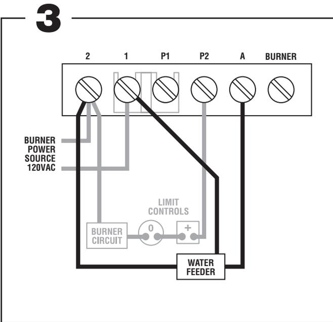
Optional water feeder connection. Connect feeder N to terminal 2. Connect Feeder H to terminal 1. Connect feeder “FEED” or “W” to terminal A. For water feeders with 2 leads, connect feeder neutral to terminal 2 and feeder hot to terminal A.
