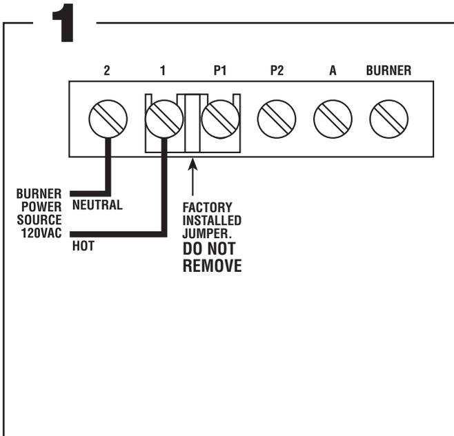
Connect input voltage (120 VAC, 60 Hz) to terminals 1 and 2.
