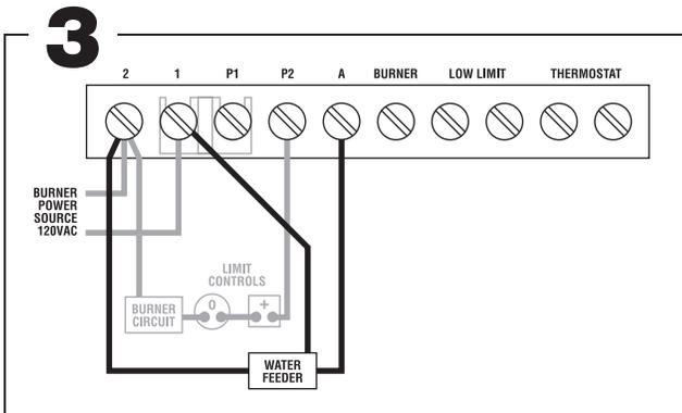
Optional water feeder connection. Connect feeder N to terminal 2. Connect Feeder H to terminal 1. Connect feeder "FEED" or "W" to terminal A. For water feeders with 2 leads, connect feeder neutral to terminal 2 and feeder hot to terminal A.
