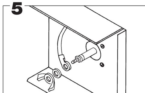
Connect the ring terminal wire lead to the probe terminal stud and secure with the lock washer and wing nut provided. With the power removed, proceed with installation and wiring according to the instructions on pages 3-4. Upon completion of wiring replace control cover.
