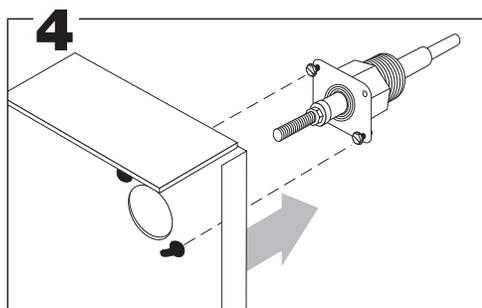
Loosen the two control cover binding head screws and remove the cover. Assemble the chassis to the probe flange and secure with the screws provided with the probe.
