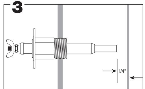
Allow 1/4" clearance from the probe to any boiler surface, tube or baffle. NOTE: Excessive use of Teflon tape to seal probe piping threads may insulate the control from boiler ground. This could result in the control not operating.
