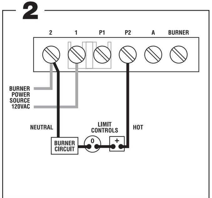
Connect terminal 2 to burner circuit neutral. Connect terminal P2 to burner Circuit in series with other limit controls. Consult boiler manufacturer instructions for proper terminal connections. Control should be wired in series with and before other limit controls.
