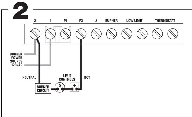
Connect terminal 2 to burner circuit neutral. Connect terminal P2 to burner Circuit in series with other limit controls. Consult boiler manufacturer instructions for proper terminal connections. Control should be wired in series with and before other limit controls.
