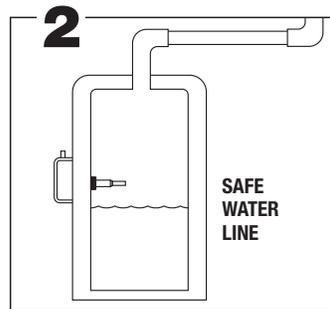
The probe may be installed in the boiler above the lowest safe water level established by the boiler manufacturer. Most manufacturers provide a suitable opening in the side of the boiler.
