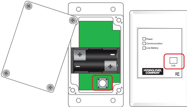
The link button on the **receiver** can also be used as a reset. If pushed, the **receiver** will revert to a power-up condition; a temperature of 75°F (24°C) will be reported until the first transmission is received (up to 10 minutes).
