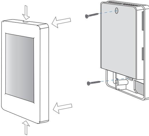
Grasp the front cover by the fingertip grips on the top and bottom of the enclosure and pull the front cover off.
