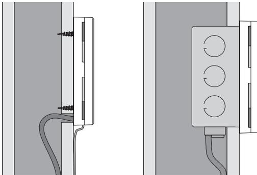
The enclosure is either mounted flush onto a wall or it can be placed onto a 2" x 4" non-conductive electrical box. The mounting holes in the enclosure accept #6 screws. Wiring to the control enters the wiring chamber through the back or bottom of the enclosure.
