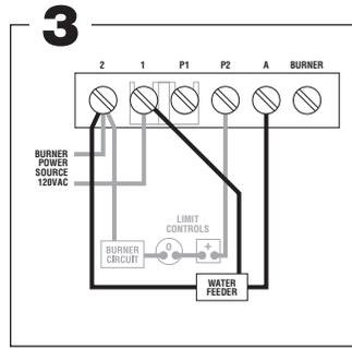
Optional water feeder connection. Connect feeder N to terminal 2. Connect Feeder H to terminal 1. Connect feeder "FEED" or "W" to terminal A. For water feeders with 2 leads, connect feeder neutral to terminal 2 and feeder hot to terminal A. **Note:** Use of a solenoid valve or McDonnell & Miller Model 101A water feeder may cause flooding and is not recommended for use with this low water cut-off.
