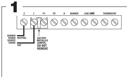
Connect input voltage (120 VAC, 60 HZ) to terminals 1 and 2.
