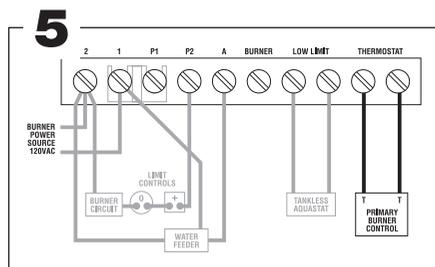
Connect "THERMOSTAT" terminals on CycleGard control to T-T terminals on burner primary control.
