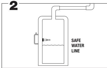
The probe may be installed in the boiler above the lowest safe water level established by the boiler manufacturer. Most manufacturers provide a suitable opening in the side of the boiler.
