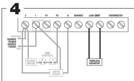
Connect "LOW LIMIT" terminals on CycleGard control to the terminals on the tankless aquastat.
