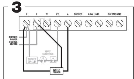
Optional water feeder connection. Connect feeder N to terminal 2. Connect Feeder H to terminal 1. Connect feeder "FEED" or "W" to terminal A. For water feeders with 2 leads, connect feeder neutral to terminal 2 and feeder hot to terminal A. **Note:** Use of a solenoid valve or McDonnell & Miller Model 101A water feeder may cause flooding and is not recommended for use with this low water cut-off.
