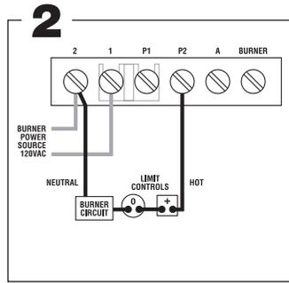
Connect terminal 2 to burner circuit neutral. Connect terminal P2 to burner Circuit in series with other limit controls. Consult boiler manufacturer instructions for proper terminal connections. Control should be wired in series with and before other limit controls.
