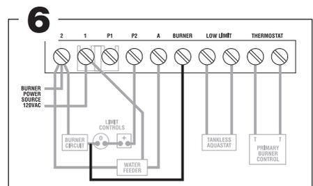
Connect "BURNER" terminal on the CycleGard control to the orange burner wire (120VAC) located under the oil burner transformer. See opposite page for schematic wiring diagram and additional SmartCycle description.
