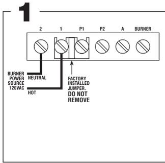
Connect input voltage (120 VAC, 60 HZ) to terminals 1 and 2.
