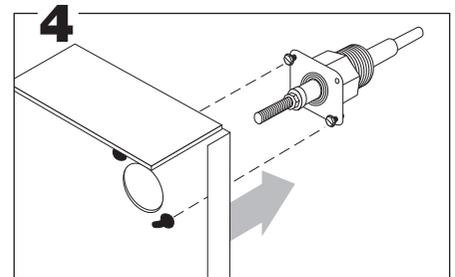
Loosen the two control cover binding head screws and remove the cover. Assemble the chassis to the probe flange and secure with the screws provided with the probe.
