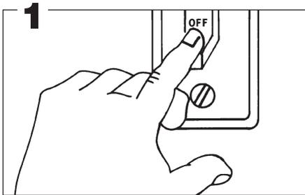
**WARNING** – To prevent electrical shock or equipment damage, power must be off during installation or servicing of the control. To prevent serious burns, the boiler should be thoroughly cooled before installing or servicing control. Only qualified personnel may install or service the control in accordance with local codes and ordinances. Read instructions completely before proceeding.
