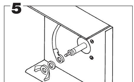
Connect the ring terminal wire lead to the probe terminal stud and secure with the lock washer and wing nut provided. With the power removed, proceed with installation and wiring according to the instructions on page 2. Upon completion of wiring replace control cover.
